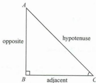
Relative to  $\angle ACB$ , BC is the **adjacent** side and AB is the **opposite** side. The **hypotenuse** is always the side opposite the right angle.
