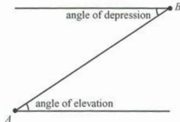
If a person stands at point  $A$  and looks up to point  $B$ , the angle between the horizontal and the line of sight is known as the **angle of elevation**.
