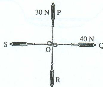
The knot at **O** does not move when the readings on **P** and **Q** are as shown.
