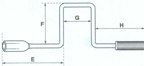
Increasing the length of one of these dimensions would reduce the effort needed by the mechanic to undo the wheel nut.
