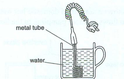
The immersion heater is placed in a cup of cold water and switched on.
