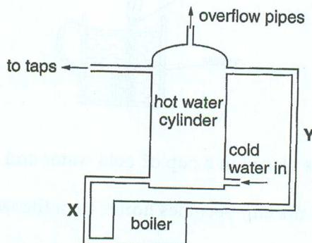
(a) On the diagram, use arrows to show the direction of water flow in pipes X and Y. [1]
