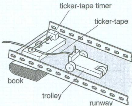
When the trolley is released, it moves down the runway, pulling the ticker-tape through the ticker-tape timer. The timer makes dots on the tape every 0.02 s.
