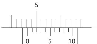
Given that the vernier caliper has a positive zero error of + 0.02 cm, what is the thickness of the wooden plank?
