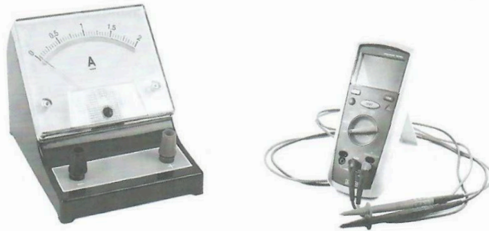
Example of an ammeter and a multimeter with ammeter function
